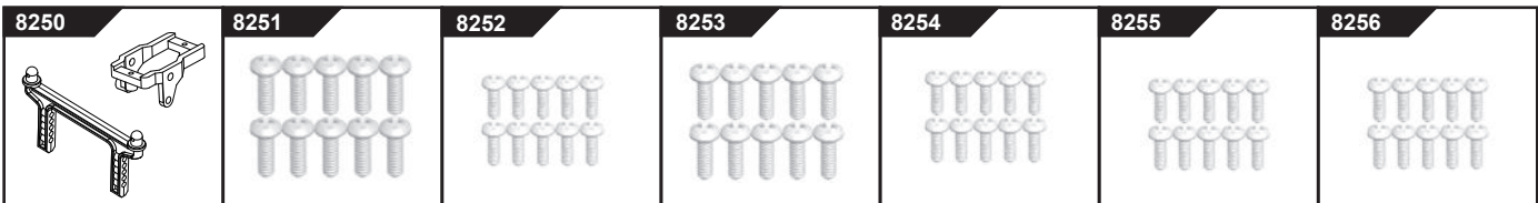
8250 Karosserie-/Servohalter Body-/ Servomount 8251 Linsenkopfschrauben Round head screws 2.5x22PB 8252 Linsenkopfschrauben Round head screws 2.5x10PB 8253 Linsenkopfschrauben Round head screws 2.5x18PB 8254 Linsenkopfschrauben Round head screws 1.7x6 PWB W4 8255 Linsenkopfschrauben Round head screws 1.7x7 PWB W4 8256 Linsenkopfschrauben Round head screws ST 2.3x6 PB
